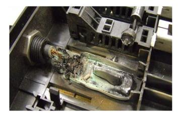
1 Inadequate Junction boxes. A bad junction box can ruin a complete solar system and the building it's installed on.
