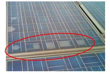
3 Delamination reduces yield and finally results in complete failure of the panel.
