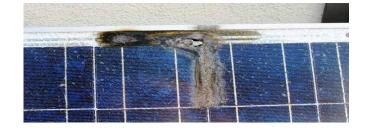
2 Incorrect soldering results in corrosion and eventually complete failure of the panel.
